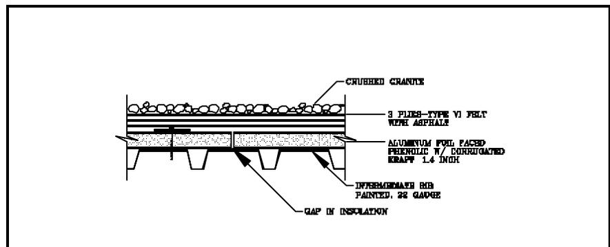
Figure 1: Project No. 1 Roof Cross Section
